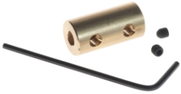
Part No. 919D1/8. In-line Coupling. 8mm-8mm Dia. 12.67mm x 24.8mm. 23g
