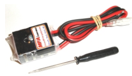
Part No. 919D2. Voltage Regulator. (6-15v DC Input. 4v-12v output). 26mm x 31mm x 15.5mm. 30g
